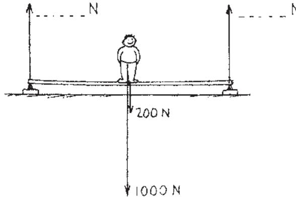
2. When Manuel moves to the left as shown, the scale closest to him reads 850 N. Fill in the weight for the far scale.
