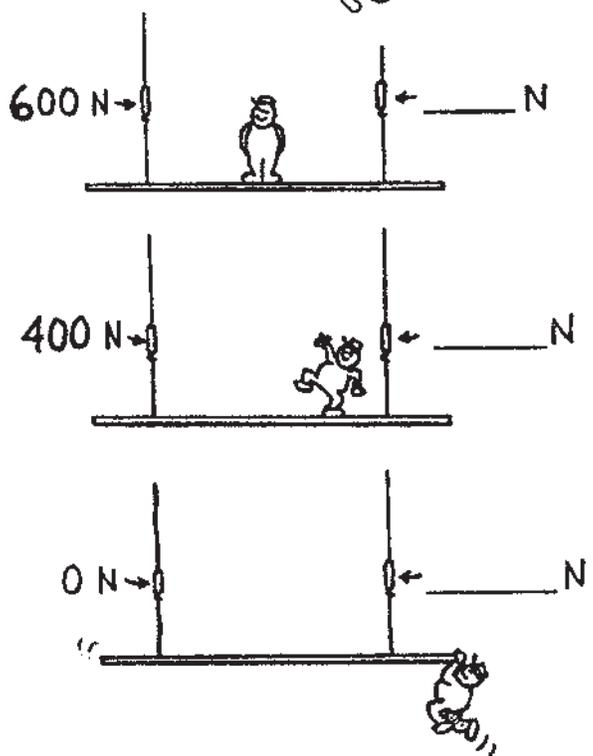
2. When Burl the painter stands in the exact middle of his staging, the left scale reads 600 N. Fill in the reading on the right scale. The total weight of Burl and staging must be \_\_\_\_\_ N.
