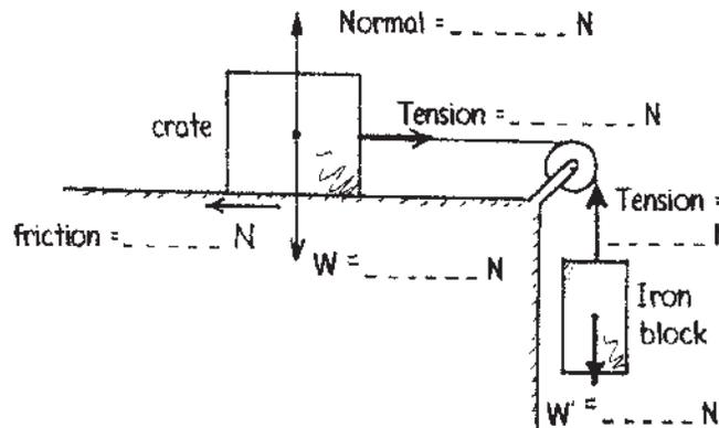
5. If the crate and block in the preceding question move at constant speed, the tension in the rope (is the same) (increases) (decreases).
